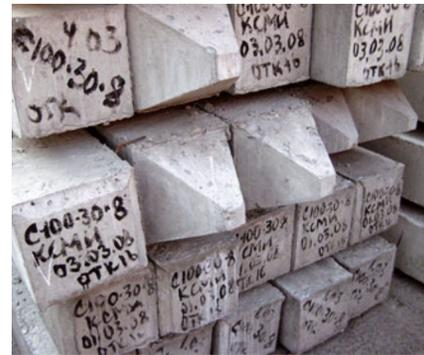
The Weckenmann experts have also designed the new bulkhead for the typical pile tips. With this, flat tips can now be produced for extension piles in addition to the pointed tips. For removal the bulkhead can be opened completely, so that the finished piles can be lifted out vertically. The result is a lower risk of accidents for the employees and no risk of damaging the finished products.
