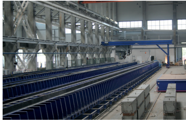
The manufacturer uses the three hydraulic twin beam formworks from Weckenmann, each 75 m in length, for the manufacture of columns with and without corbels, as well as prestressed girders and downstand beams.
