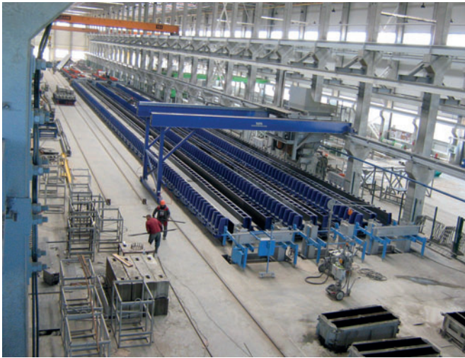
The manufacturer uses the three hydraulic twin beam formworks from Weckenmann, each 75 m in length, for the manufacture of columns with and without corbels, as well as prestressed girders and downstand beams.
