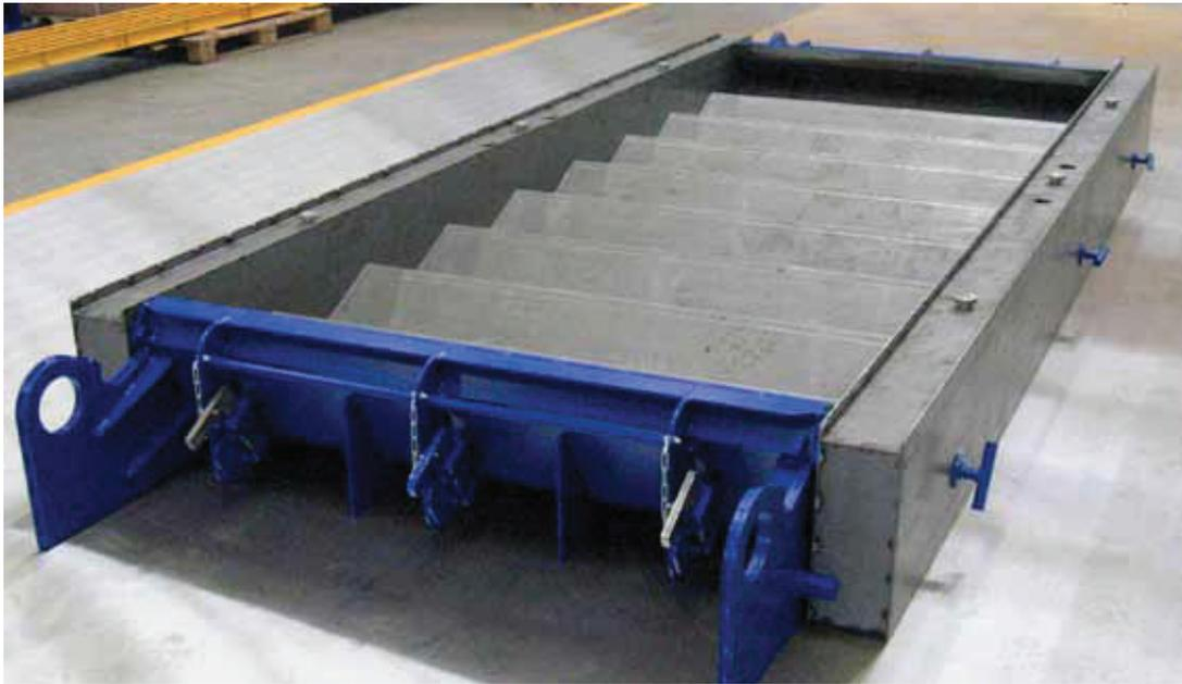
The staircase formwork of Weckenmann is perfectly suitable for the flexible production of stairs on stationary tables or on pallets in a circulation system
