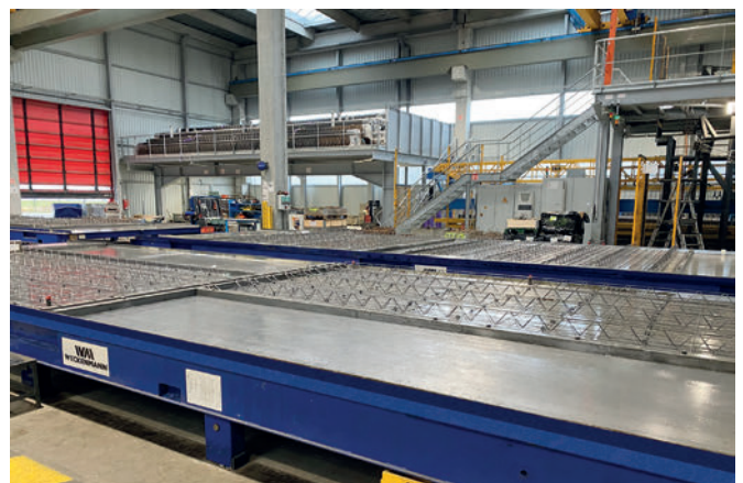
Weckenmann pallets (60 pallets included in delivery, of which 12 pallets with 60 mm high edge formwork and 48 pallets with edge formwork of 70 mm in height) Insertion of reinforcement and accessory formwork pallets with A-formwork and integrated magnets
