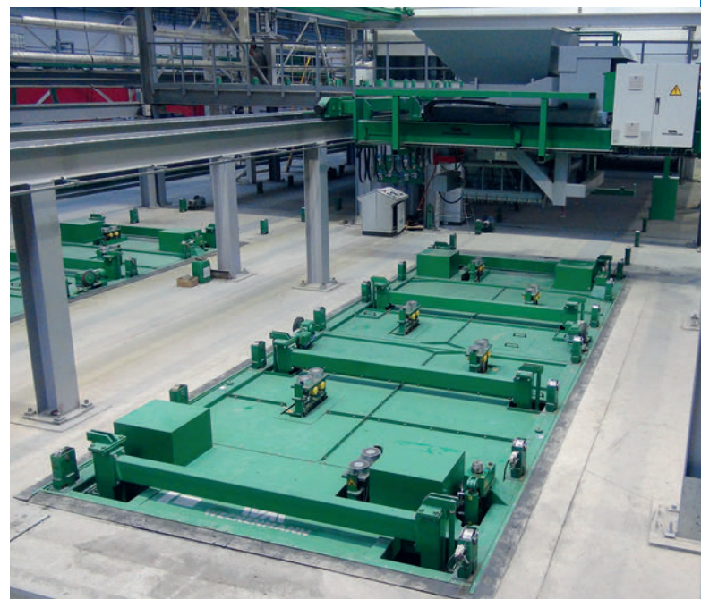
Combined shaking and vibrating station
