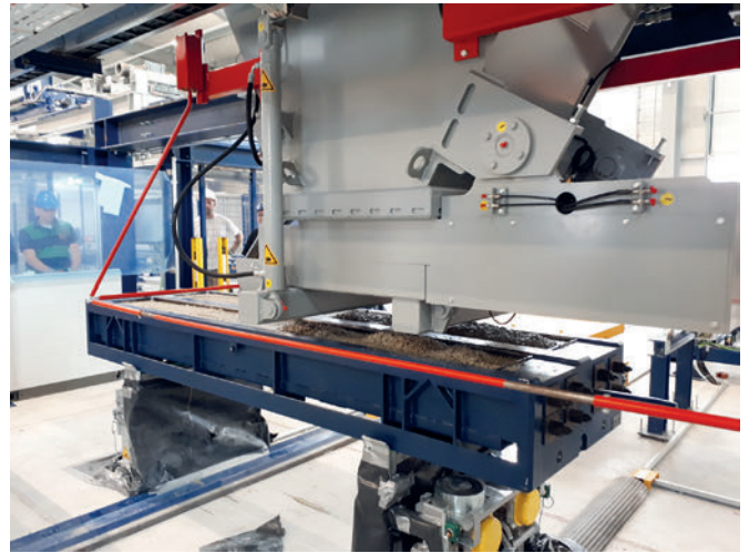
MagVib in point sleeper production
