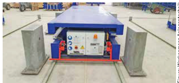
Front view of the run-off carriage with the hydraulic lifting platform on which the stacks of floor slabs are placed
