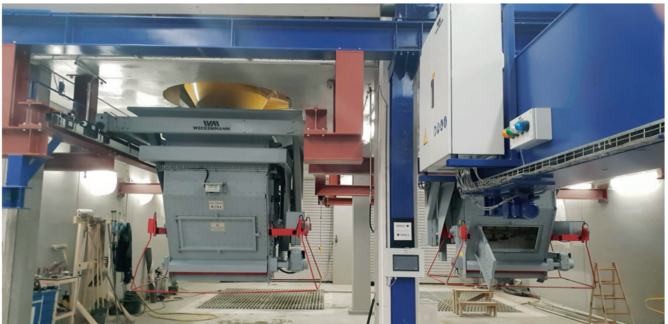
Concrete distributor with two buckets
