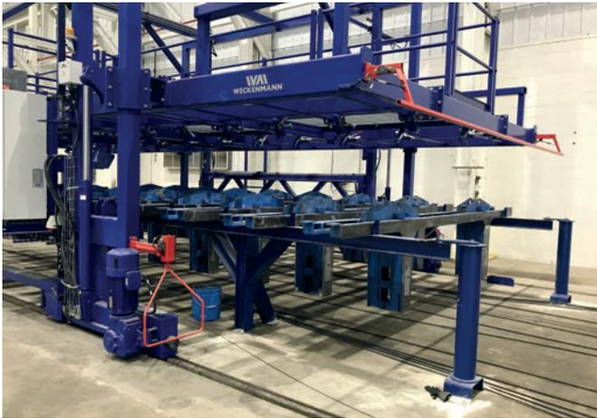
Utility Cart (Strand pulling and bulkhead placing)
