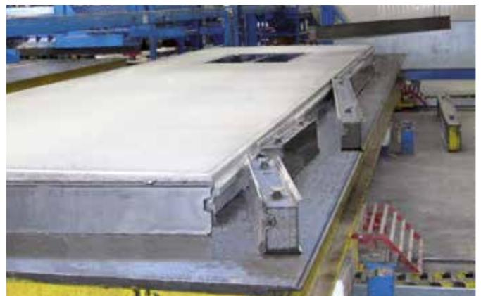
in the production of a solid wall panel with chamfer design and cast joints
