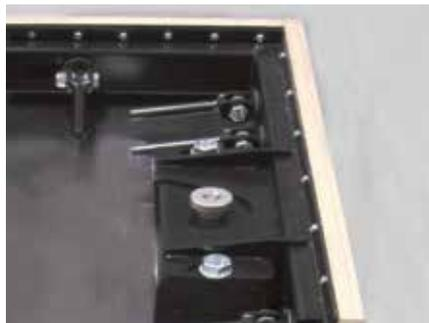
The MagnetBox serves as a carrier for Weckenmann system shuttering
