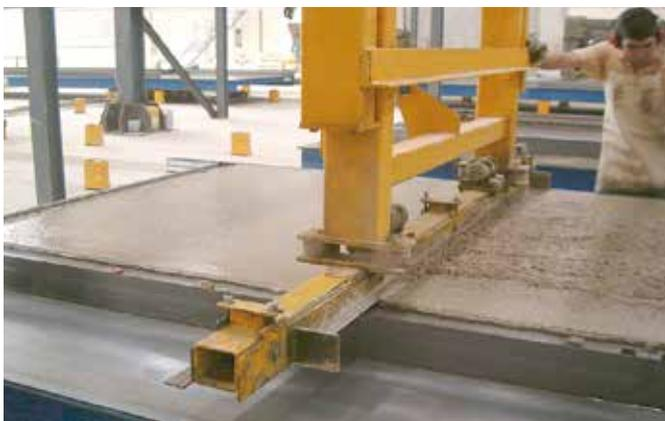
also suitable for the mechanical levelling of the finished part surface by machinery
