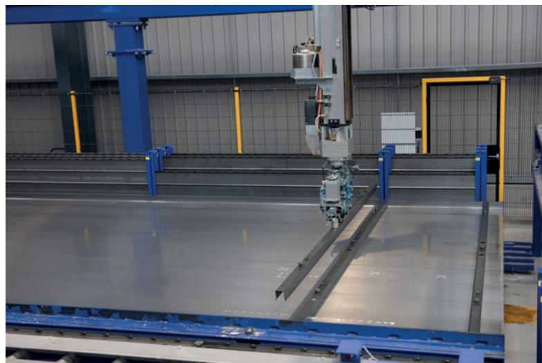
Shuttering robot at Keegan Precast Ltd.
