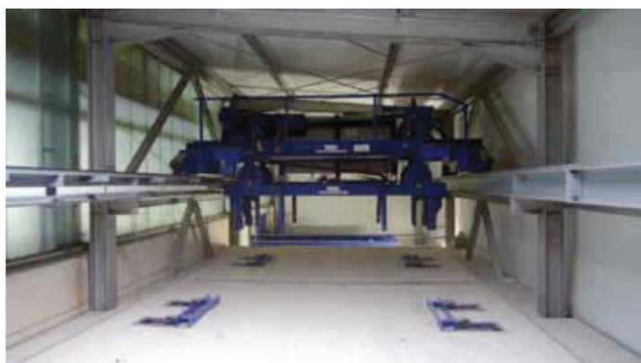
View into the new curing chamber with fully automated stacker crane
