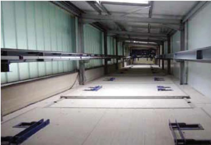
five individual compartments. If a compartment is fully used, it is automatically closed by the stacker crane. The minimum curing time is exactly controlled by the system. Once this period elapses, the crane retrieves the molds, and then they are fed again into the circulation via a heavy-duty roller conveyor.
