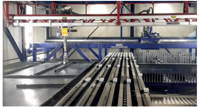
The formworks from the magazine are fed to the formwork robot on new roller conveyors.
